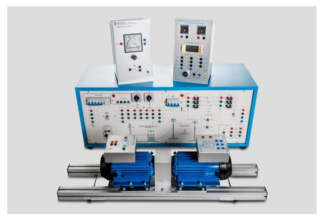
This laboratory simulates a real life generation, transmission and utilization system based on standard electrical machines, instruments and a simulated transmission line.
